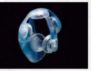
Rocco Giovanonni's Inmergo headphones use liquid rather than air to carry sound, improving current bone-conduction audio technology<sup>31</sup>. The technology could be applied to deliver rich audio for people with hearing loss and for sound-therapy or virtual reality experiences.
